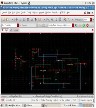
Fig.4 proposed schematic of high pass filter
