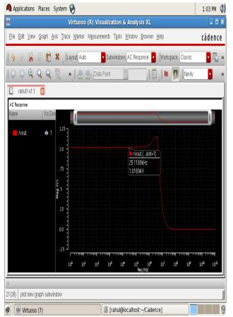
Fig.3. response of low pass filter.
