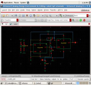
fig.6.proposed schematic of band pass filter.
