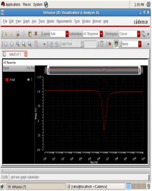
Fig.9 response of band reject filter.
